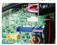
\*\*\* Indoor PCB drain pump connector (Check input of DC 15V) (Marked as CN\_DCDRAIN)
