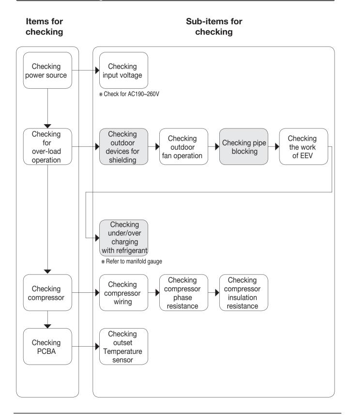
CH 35 (Discharge pipe overheating error of Inverter)
