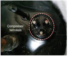
Measure the line resistance between the compressor terminals.
