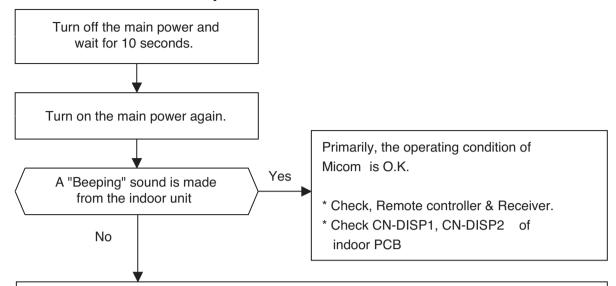
Check the voltage of power supply (AC220V/AC240V, 50Hz) and check for the following :
