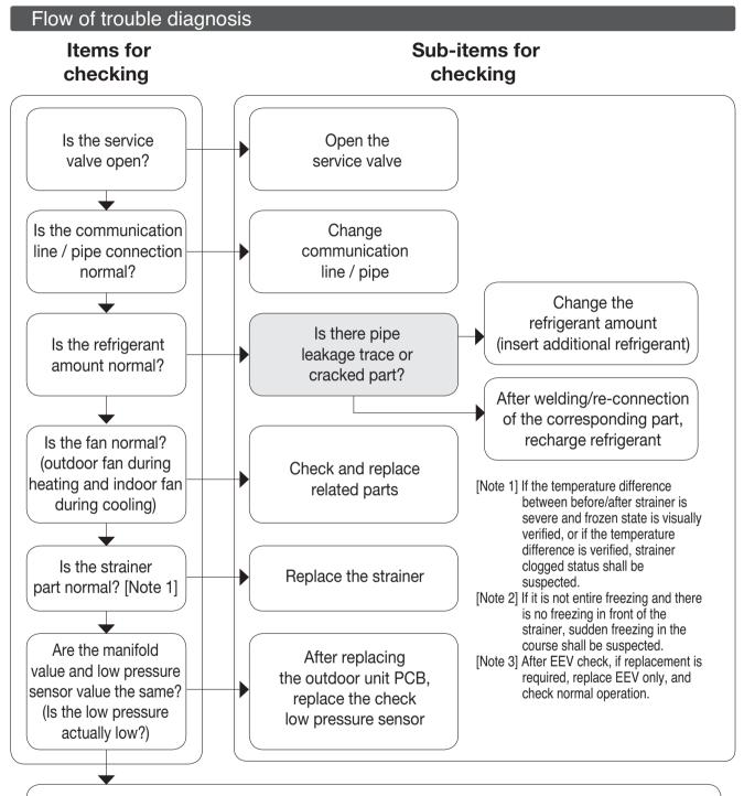
Check indoor/outdoor EEV / check indoor/outdoor unit PCB / check indoor/outdoor unit installation environment
