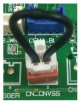
Connector with capacitor in CN FLASH and CMN CNVSS
