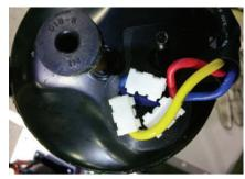
Check whether the compressor wires are properly connected with U, V, and W.
