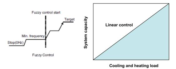
Inverter linear control as cooling and heating load increasing
