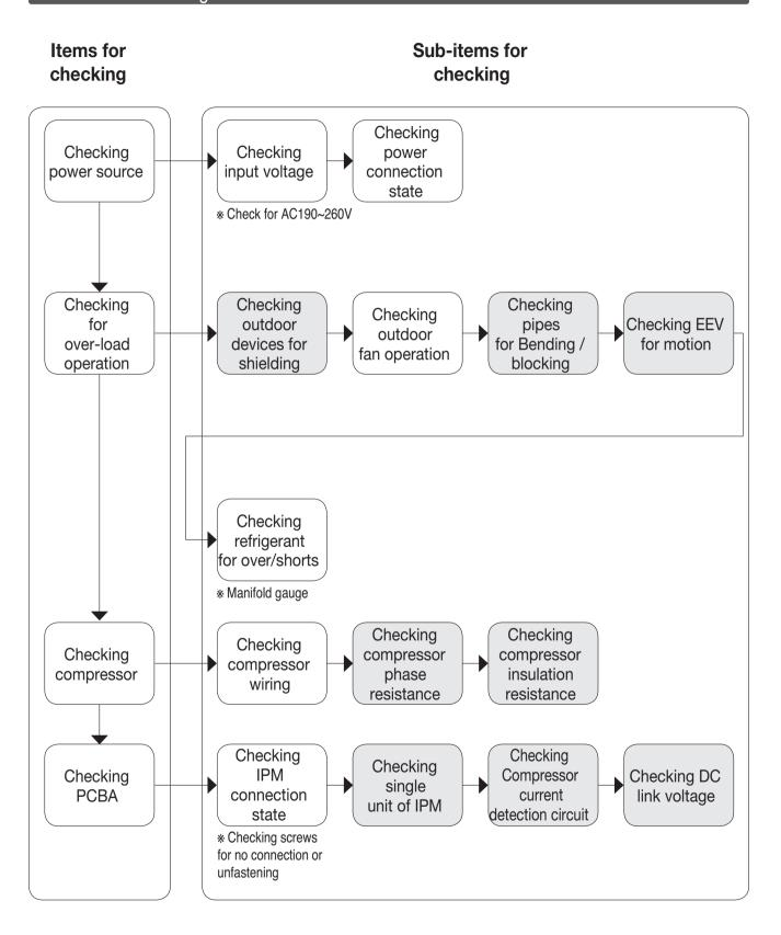
CH 32 (Discharge pipe overheating error of Inverter)
