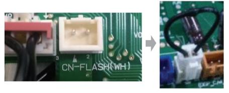
[Connector with capacitor in CN\_Flash\_Writer or CN\_Flash]
