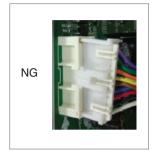
② Damage of wire coating: Interference with wires or wire coating damage with chopping
