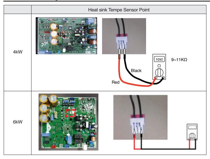
CH 65 (Heat sink Temperature Sensor Open/Short)
