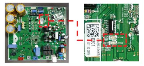
CH 05/53 (Indoor/Outdoor Device Communication Error) → Detection by indoor devices
