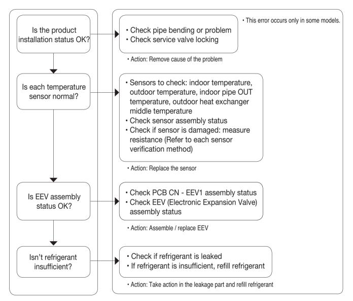
! Caution : Before checking PCB or various outdoor unit electricity flowing parts, start the checking 3 min. after power cut off. If it is measured in power supply stand by state, check the tester's measurement mode and be careful of the short circuit with parts other than the measurement part.
