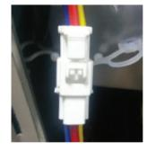
[Picture of normal compressor wiring]
