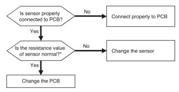
\*\* In case the value is more than  $100k\Omega$  (open) or less than  $100\Omega$  (short), Error occurs
