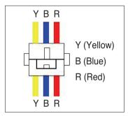
Check whether the PCB wires and compressor wires are connected in the same colors.
