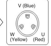
\* The wiring direction is CCW. (counter clock wise)
