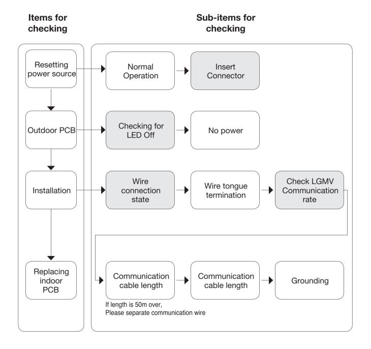
CH 05/53 (Indoor/Outdoor Device Communication Error)  $\rightarrow$  Detection by indoor devices
